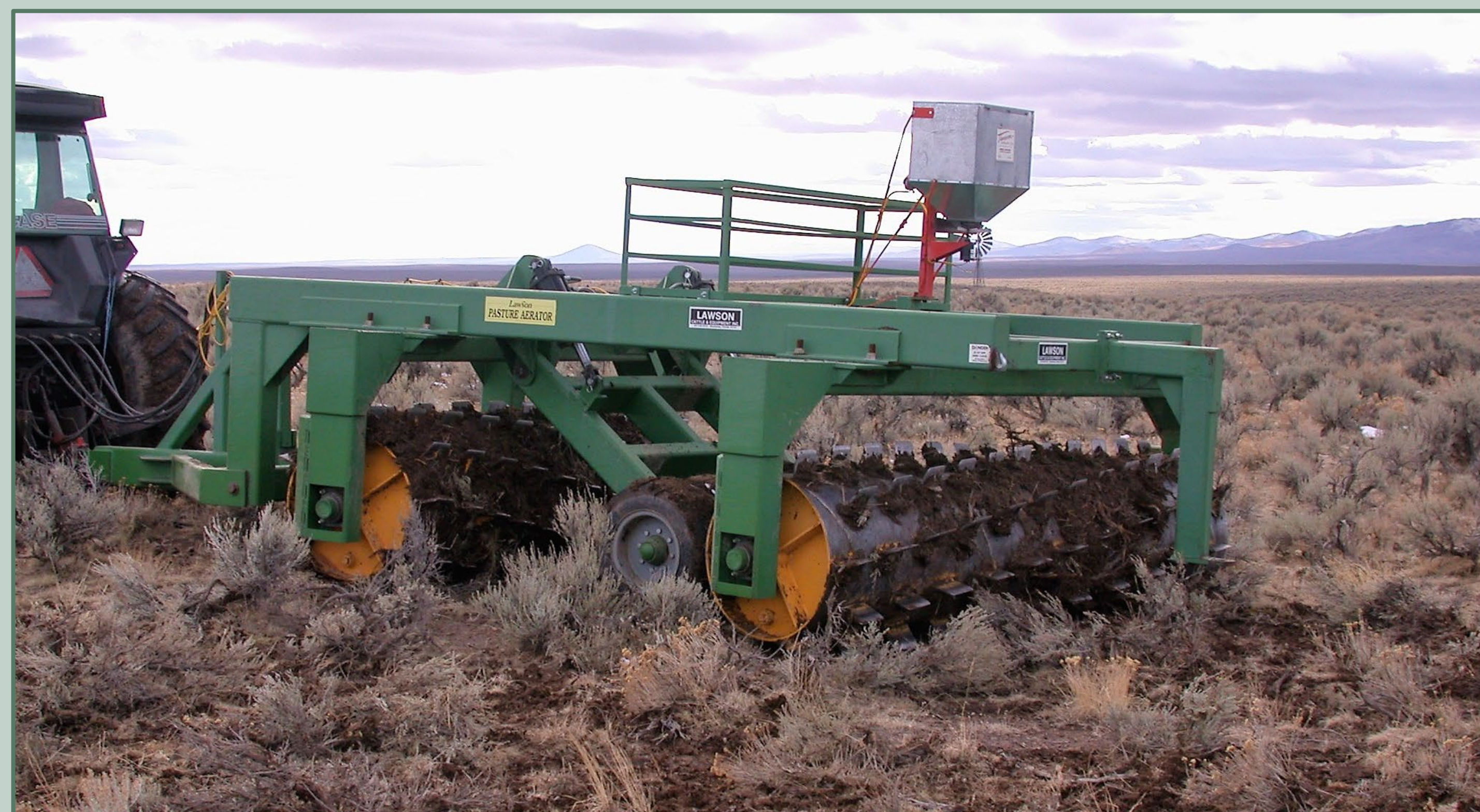
Figure 1. Lawson Aerator is a tool that can be used on rangelands to improve stand decadence, herbaceous forage and edge effect for wildlife.
